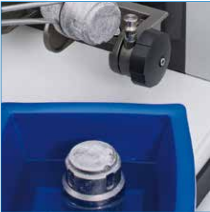
Cooling a jar in liquid nitrogen
