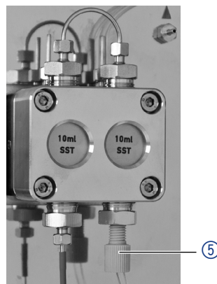
Fig.8 Solvent line on pump head
