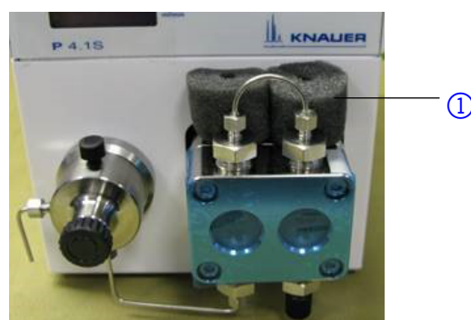
Fig.5 Transport protection between the ends of the pump capillaries and the housing
