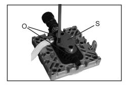
Loosen the clamping brackets (S) on the valve heads (O).
