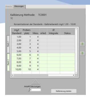
The "Measurements" tab opens automatically, where you will see a table showing the concentrations entered. The table is divided into Rack 1 and Rack 2. In Rack 1 are the first 5 standards and Rack 2 is the next 5. When the first 5 standards have been measured, the rack must be replaced so that the remaining standards can be measured. A rack change notice appears.
