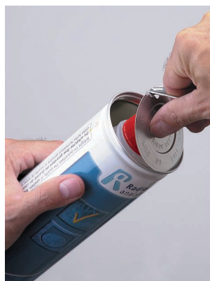
pH buffers can be stored in sealed cans for up to 2 years.
