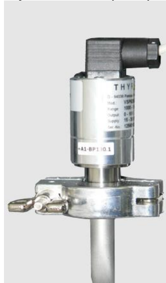
Fig. 13: Vacuum sensors of different manufacturers
