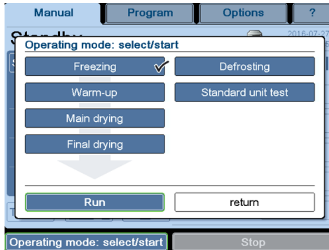
Fig. 28: Dialog box "Operating mode: select/start" (The version of the dialog box that is displayed depends on the equipment of the freeze-dryer.)
