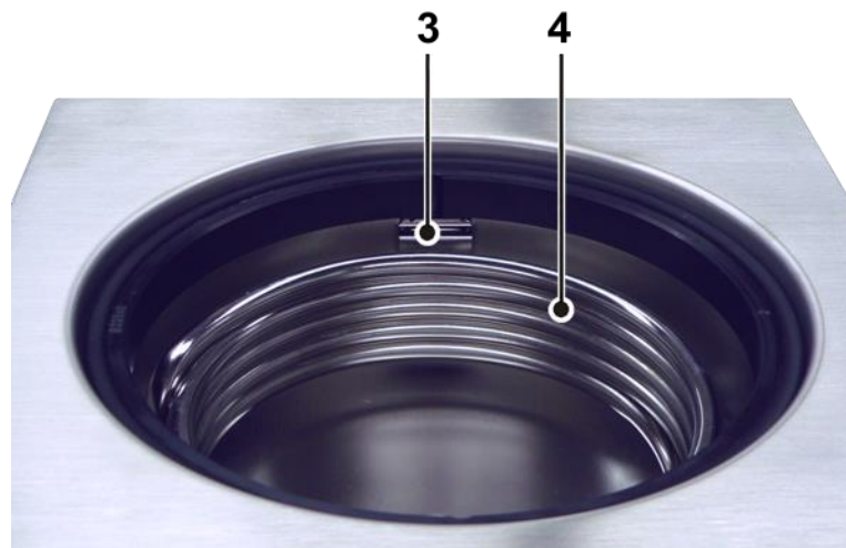
Fig. 48: Ice condenser chamber
