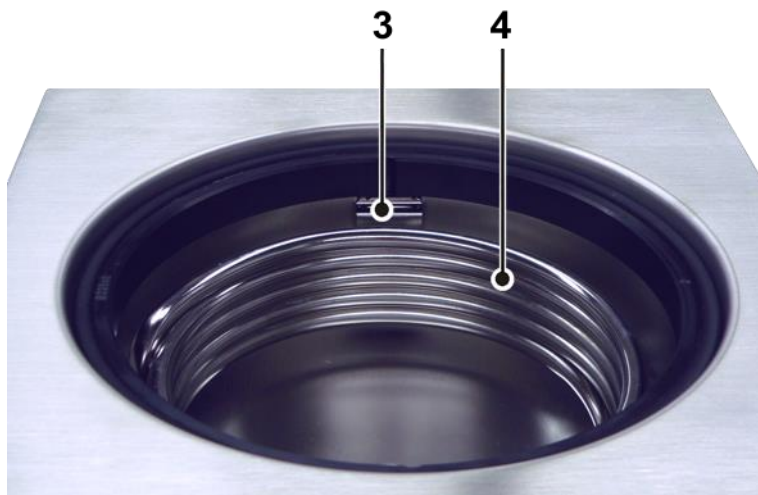
Fig. 2: Ice condenser chamber
